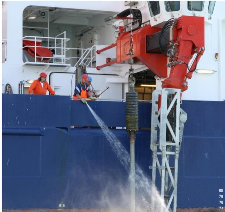
Fig 2.4.2: During station works within Disko Bay the Gravity-Corer was equipped with a 18 m long steel tube.
