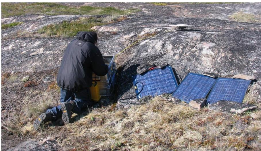
Fig. 2.10.3: Example for the setup of a GPS station at the site NSFC. On top of the rock outcrop, the antenna is mounted. The GPS receiver and the accumulators are stored in an aluminium box, solar panels are used for the power supply.
