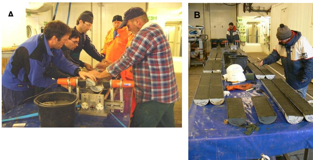
Fig. 2.5.1: (A) Plastic liner from the Gravity-Core splitted using a core cut device. (B) Splitted gravity core with cleaned sediment surface.
