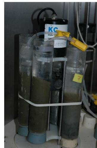
Fig. 2.7.2: a) Microscopy: Looking for live foraminifers in mud at in situ temperature. b) Flux: Set up used for measuring bacterial N-transformations and exchange of nutrient between the surface sediment and the overlying water.
