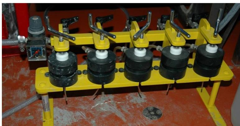
Fig. 2.7.3: Porewater presser: Equipment used for extracting porewater from sediments.
