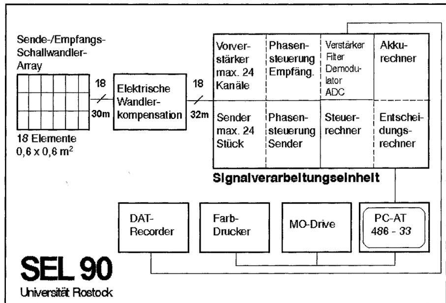
Fig. 2.5.2-1 Configuration of the sediment penetrating echosounder SEL90
