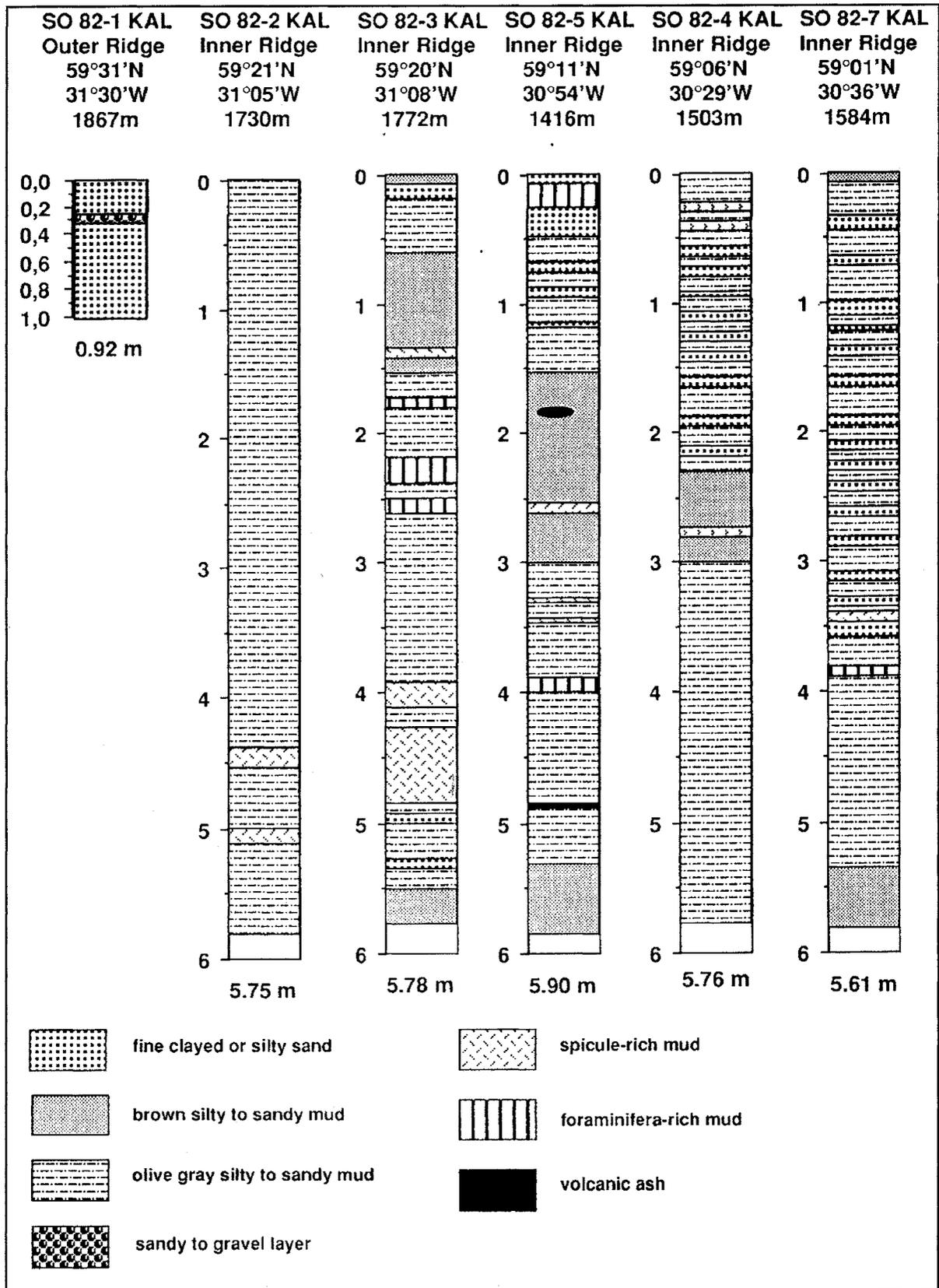
Fig. 3.5.2-2 Lithology of the giant gravity cores
