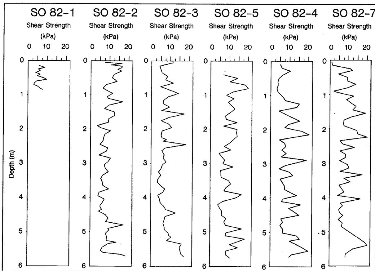
Fig. 3.5.3.-1 Shear strength of the giant gravity cores
