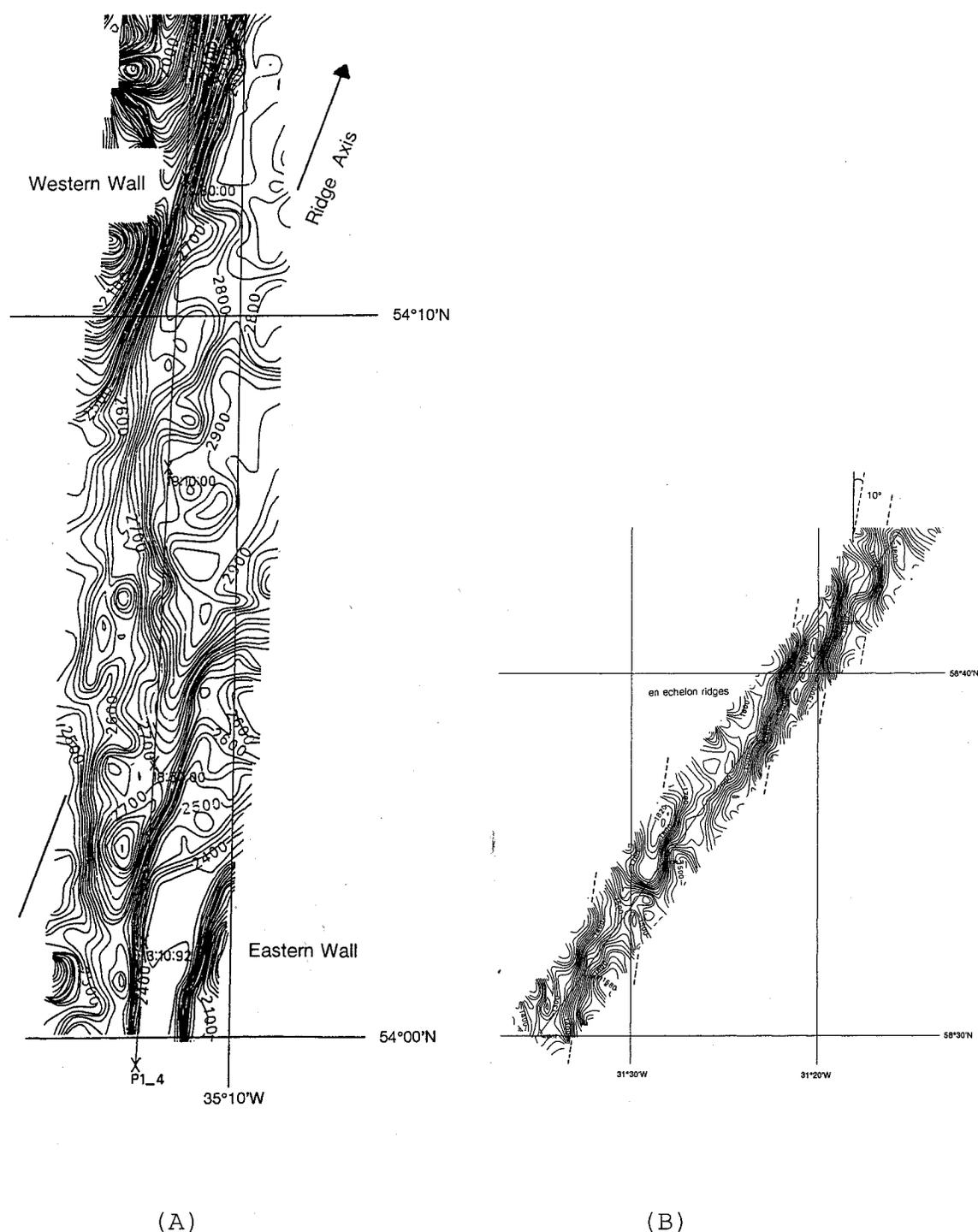
**Fig. 2.5.3.-2 Hydrosweep stripes of the Reykjanes Ridge crest, 20 m contour intervall. (A) The southern segment is characterized by a median valley and bounding rift mountains, the valley is dominated by a tectonic graben. (B) En echelon ridges, trending perpendicularly to the spreading direction, but are oblique to the strike of the axis of spreading are located in the rift valley floor of the northern segment.**
