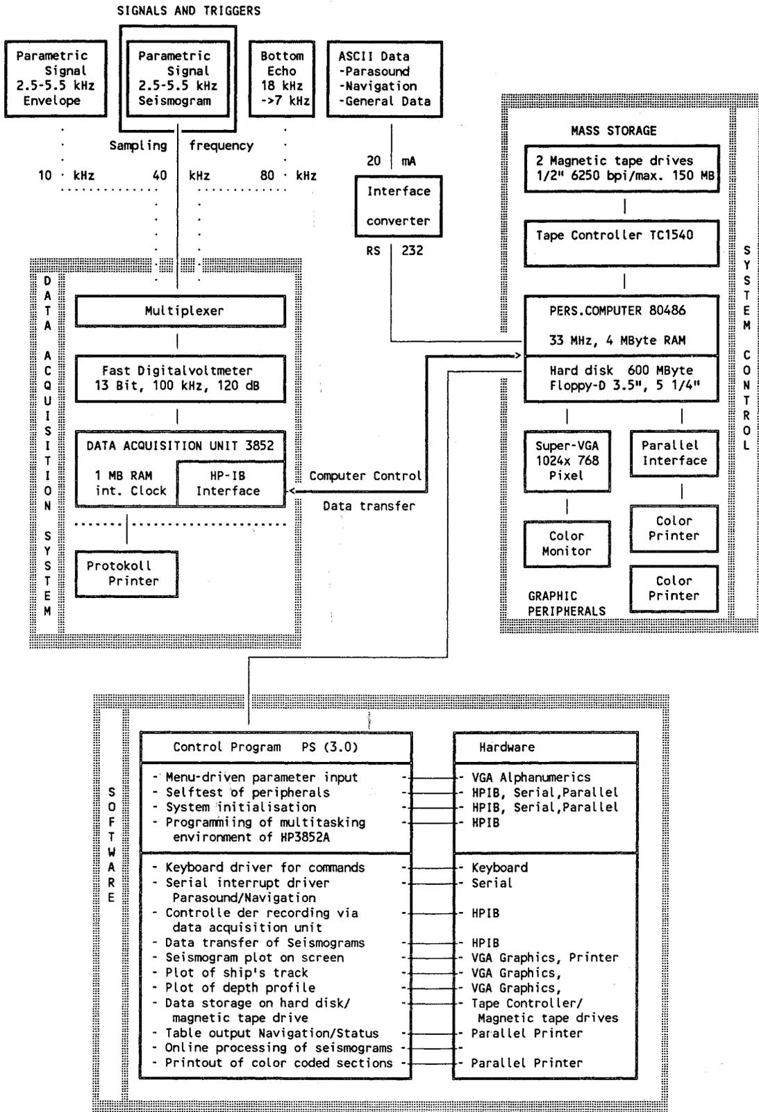
Fig. 2.5.1.-1 Hardware concept and software components of the Paradigma System (PARAsound DIGitizing and Multichannel Analysis System)
