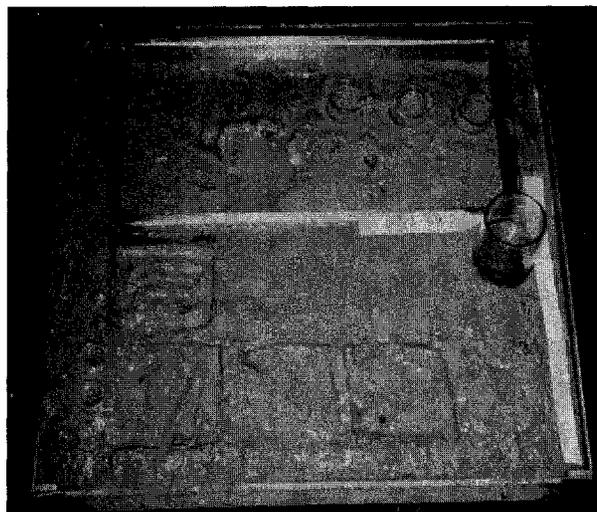
**Fig. 3.5.2.-1 Sub-sampling of the large box core**
